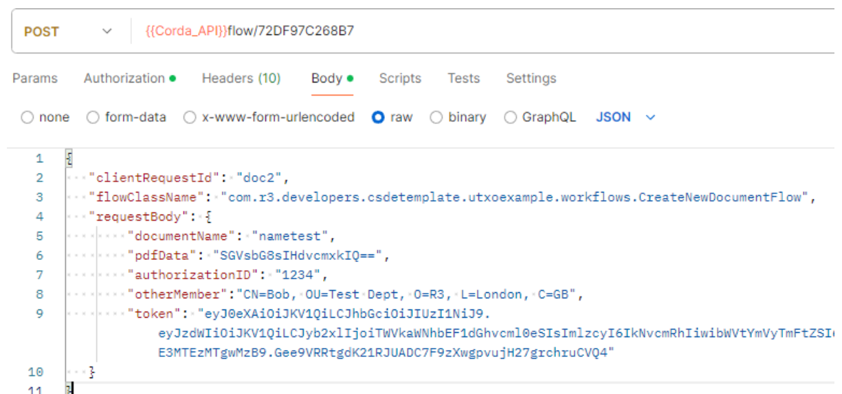
Figure 3.1: Example of a HTTPS request of the creation of Documents in Postman to the Corda application
