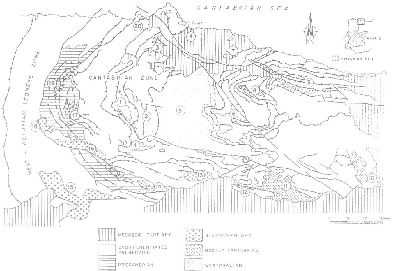
Figure 1. Schematic geological map of the Cantabrian Mountains showing the location of the most important coalfields: 1-Teverga-San Emiliano; 2-Quirós; 3-Santiforme-Naranco; 4-La Camocha, 5-Central Asturian; 6-Coballes; 7-Sueve-Libardon; 8-Sebarga; 9-Cabrales; 10-La Pernía-Barruelo; 11-Guardo-Valderrueda; 12-Sabero; 13-Ciñera-Matallana; 14-La Magdalena; 15-El Bierzo; 16-Villablino; 17-Carballo; 18-Rengos; 19-Cangas-Tineo; 20-Arno (adapted from 13).
