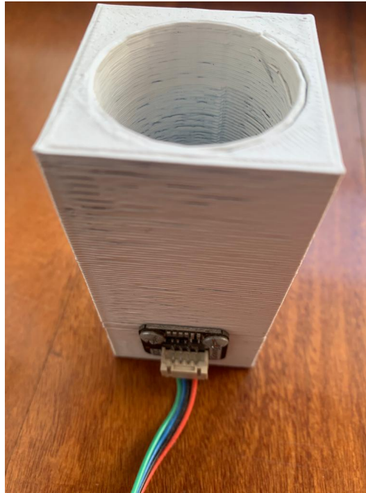
Figure 4.10: Assembly of the sensor in the system
