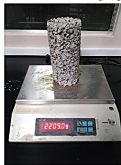
Figure 7. Pervious concrete weighing with STT
