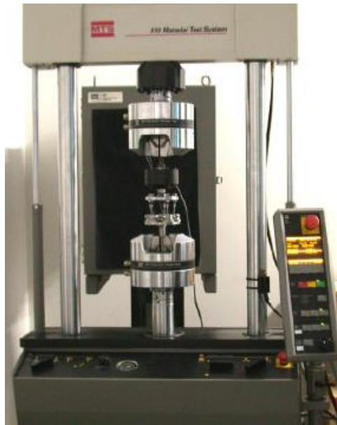
Figura 5- Material Test System – MTS 810. (Ref. http://www.upc.edu/sct/documents equipament/d_77_id-412.pdf ).
