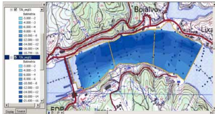
Figure WP13.4. TIN formatted surfaces for the first three model segments and respective legend.
