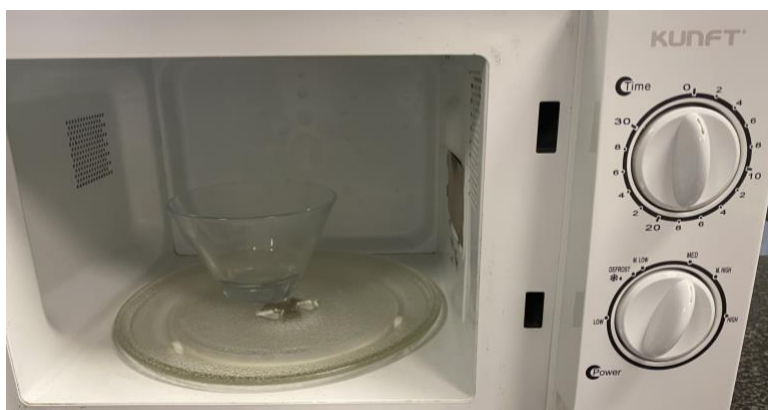
Figure 17 - Heat tempering using a microwave, selecting 450-500W power for 4 minutes
